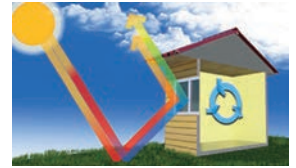
Low-E reduces solar heat gain by diffusing radiation coming from the sun.
